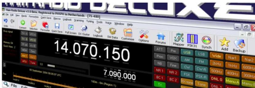
One of the first features you set up is CAT control so that your Digimode software can set and get the frequency and mode of your radio.
